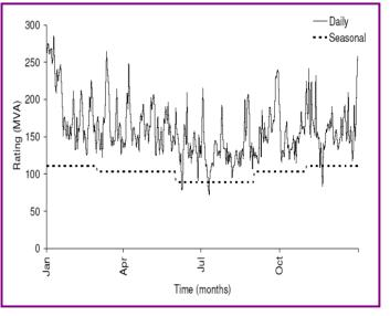
weather enhanced rating system for the main interconnected transmission system for
