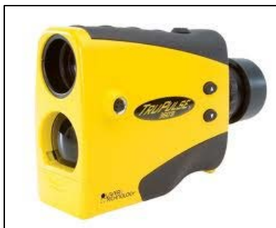
Figure 5-5: 'TruPulse' laser measurement tool for identifying clearance to conductors from ground/objects
