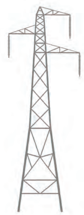
132kV Steel Lattice Tower PL1 20 metre height
