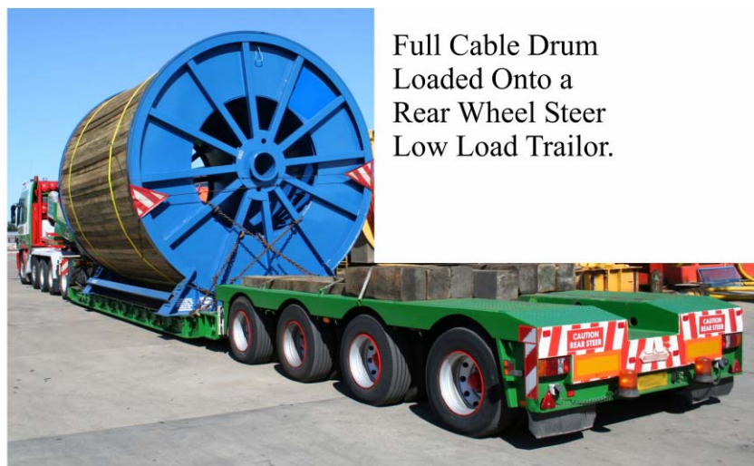
Figure 2-11 Cable Drum Load Transversely onto a Trailer
