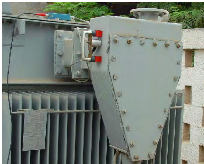
Figure 2.7 Example of externally applied acoustic sensor
