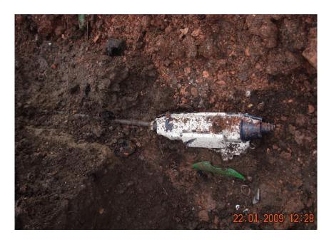
The above image highlights a low voltage cable with a straight joint attached. An operative took a hacksaw and severed the cable which was attached to the ScottishPower network.
