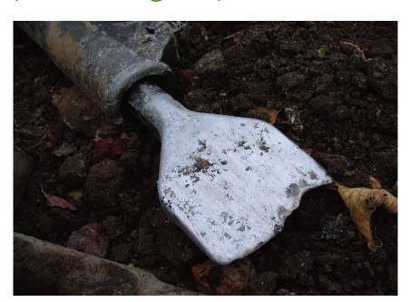
The above Image highlights a damaged spade tool on a pneumatic gun which has come into contact with a low voltage cable.
