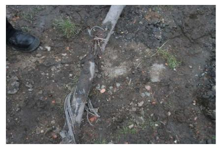
The above image highlights the consequences of driving a 5m length metal earthing rod into the ground at a primary electrical sub-station.
