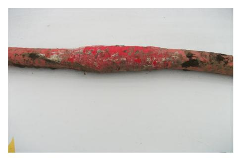
The above image highlights a section of HV cable found with red insulating tape covering the point of damage. The operative who placed the insulating tape around the cable, not only placed themselves in danger, they left a dangerous situation for operatives excavating at this location at a later date.
