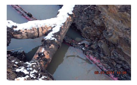
The above image clearly shows an underground HV Coral cable damage.
