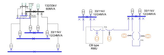
33kV networks tend to radiate outwards from 132kV bulk supply points, similarly 11kv networks tend to radiate outwards from primary substations. Historically companies will have tapered the network cables, as the cable travels further form the supplying transformer, but more recently uniform (standardised) cables have been employed.
