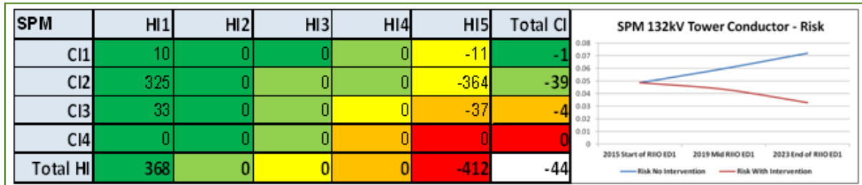
Figure 6: 132kV OHL Conductor Health and Criticality Indices with intervention during ED1
