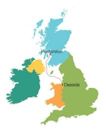
The Western Link will transmit up to 2,200MW (megawatts) of direct current (DC) electricity from Scotland to England and Wales, bypassing the bottlenecks on the existing national transmission network. Because the electricity we use in our homes, schools and offices is alternating current (AC), we need a converter station at each end of the link to change the electricity from DC to AC before we can use it.
