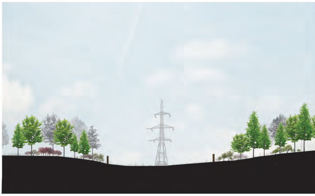
Section 1 Illustrating the treatment proposed to the wayleave corridor alongside the line as it emerges from the Loch Ard Forest and crosses Muir Park. The section shows the proposed fence line in relation to the edge of the proposed planting. It is proposed to leave a swathe of land, of varying width and design, between the woodland edge and the fence line to encourage natural regeneration within this area and a feathering out of the woodland edge to create a more natural 'edge zone' with increased biodiversity value. The woodland edge will vary in design along the wayleave in accordance with the principles outlined below.
