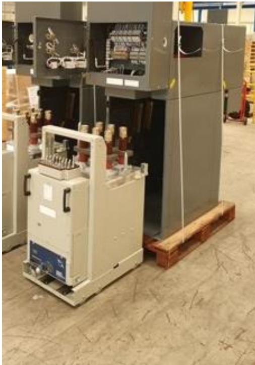
Figure 34: 11kV Primary Switchgear Vacuum retrofit (Nil) & 11kV SF 6 Primary Switchgear (~0.5kg SF 6 )
