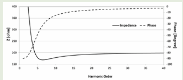
Figure 2: The impedance frequency sweep of 132kV C-type harmonic filter tuned at 245Hz
