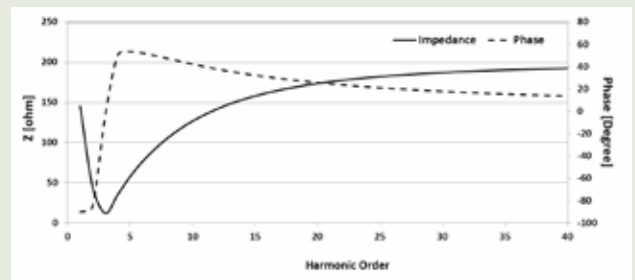
Figure 1: The impedance frequency sweep of 33kV C-type harmonic filter tuned at 147Hz
