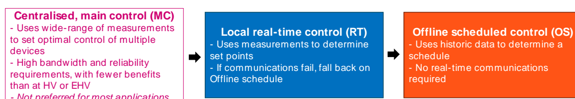
Figure 2.2 Hierarchy of control from most sophisticated to most robust, covering centralised main control (MC), local real time control (RT) and offline scheduled control (OS). Most D-Suite functionality can be achieved using only RT or OS control, and so MC is not preferred for most D-Suite applications.
