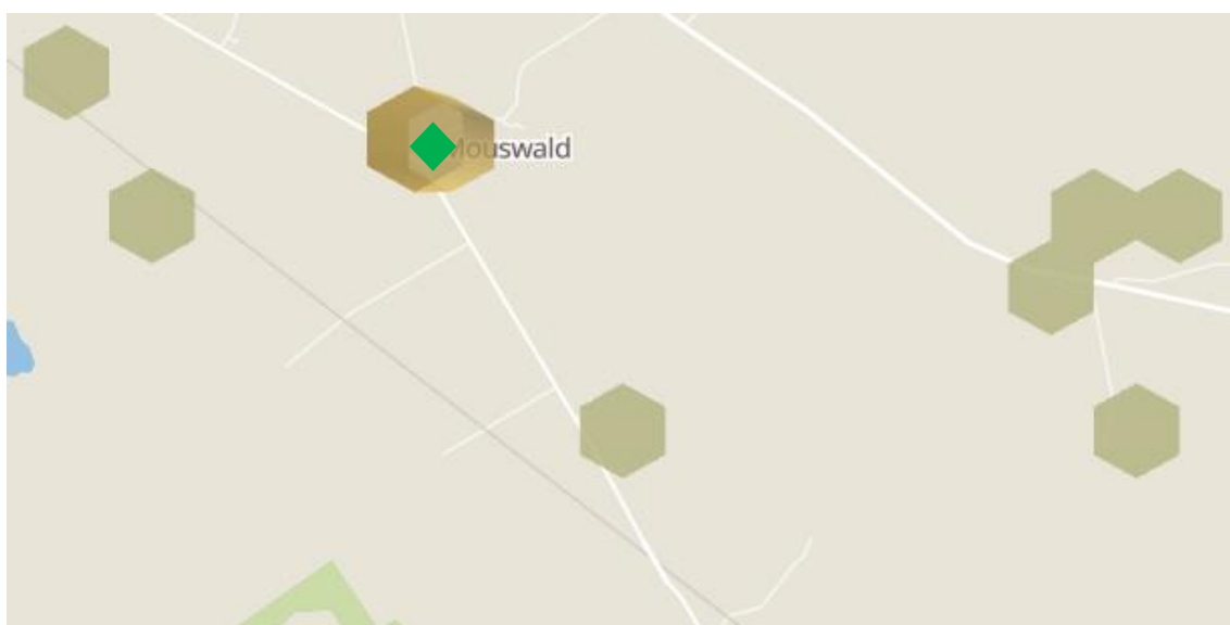
Figure 22. High-level image of HV network in Dumfries, with the higher hexagons highlighting the parts of the network that are expected to have issues due to future LCT penetration. The green diamond marks where SPD-RU is located.
