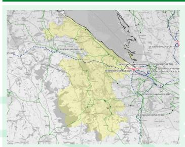
The Brymbo-Hawarden-Holywell 33kV network group supplies the area in North Wales around Brymbo, Flint, Hawarden and Holywell. It is fed from the Connah's Quay-Pentir- St. Asaph 132kV group from long overhead line circuits. The group supplies ca. 26,300 customers, including two major industrial sites.
