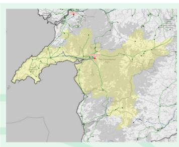
The SP Manweb (SPM) network in North Wales around Maentwrog, Porthmadog, Pwllheli, Criccieth, Blaenau Ffestiniog, Harlech and Morfa Nefyn is supplied from Trawsfynydd Grid Supply Point (GSP). The 132kV network group secures Maentwrog/Four Crosses 33kV group supplying ca. 42,000 customers which includes several recreational/tourist destinations spread across the network.
