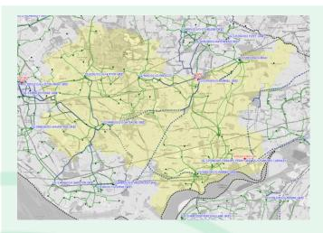
Prescot 132/33kV grid substation is supplied from within the Rainhill 132kV GSP group via 2 x 60MVA Grid Transformers (GTs) and is operated split with the 33kV bus section run as a normal open point. The 'A' board supplies the Bold/Prescot/Widnes 33kV grid group, which supplies ca. 47,000 customers. The 'B' board supplies the Gateacre/Huyton/Kirkby/Prescot 33kV grid group, which supplies ca. 68,000 customers.
