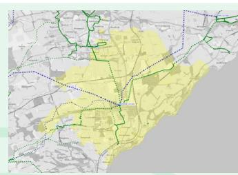
Redhouse 132/33kV Grid Supply Point (GSP) is located in the Central and Fife district of SP Distribution, providing supplies to ca. 23,000 customers via four primary substations. The Redhouse network is a mixture of urban and rural environments, comprising a mix of underground cable (UGC) and overhead line (OHL). Redhouse GSP is interconnectable at 33kV with Leven GSP, Glenniston GSP and Glenrothes GSP.
