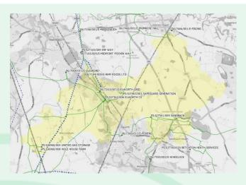
The Sandbach primary substation comprises of a single 7.5MVA 33/11kV transformer, supplied from 4 x 33kV circuits in theCrewe/Coppenhall/Radway Green/Whitchurch grid supply group. The Sandbach primary network group supplies ca. 3,400 customers with a mix of domestic, industrial and commercial customers. The 11kV group network is normally operated split from the adjacent primary group network.
