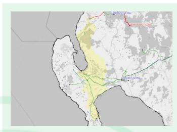
The Stranraer demand group supplies ca. 6,000 customers and is geographically located in the Dumfries and Galloway region of SP Distribution (SPD) licence area. It is supplied by Glenluce Grid Supply Point (GSP), via two long 33kV overhead line (OHL) circuits (14 and 15.5km).
