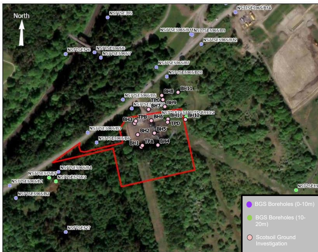
Figure 4-1: BGS Borehole Location Plan
