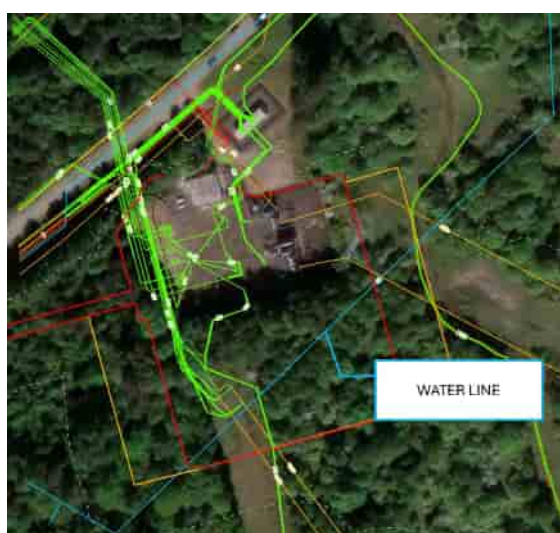
Figure 7- Existing utilities around Cumbernauld Substation
