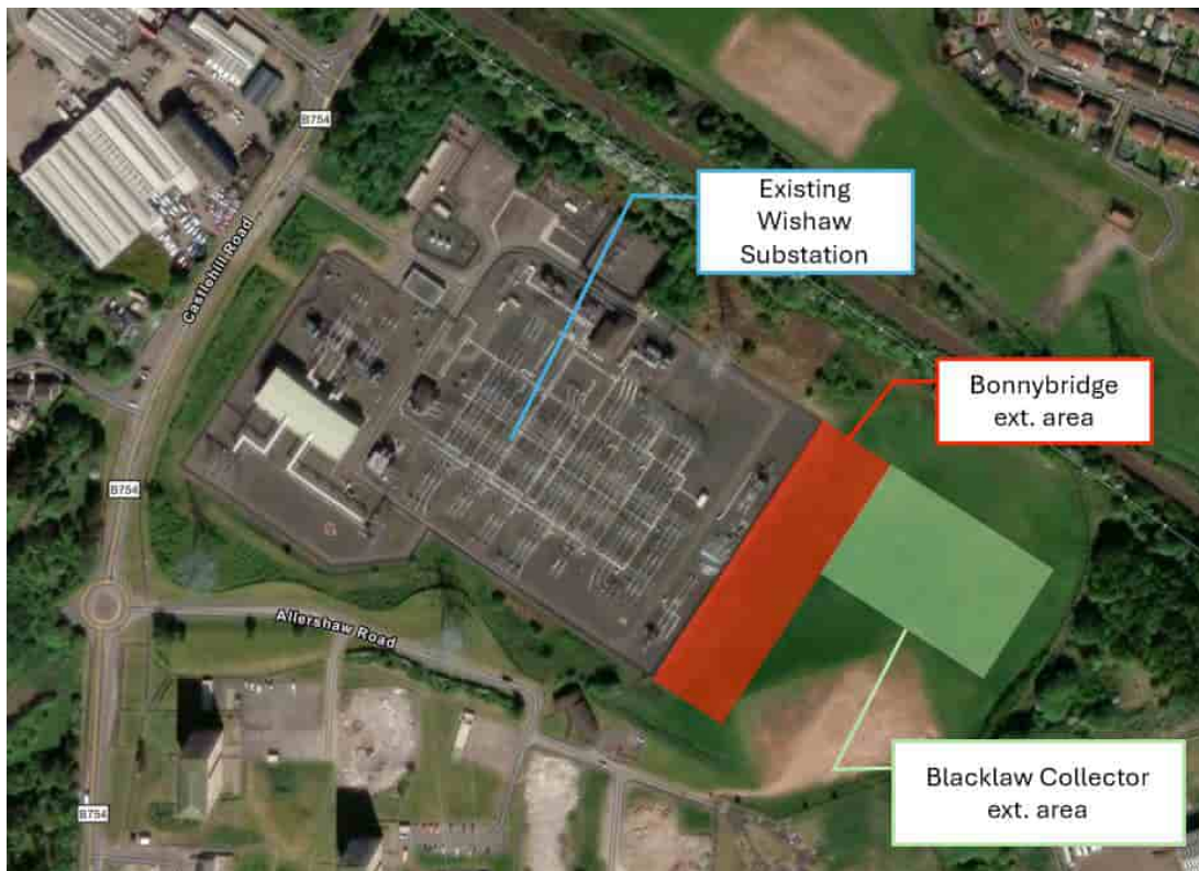
Figure 1- Overview of proposed expansion and existing substation
