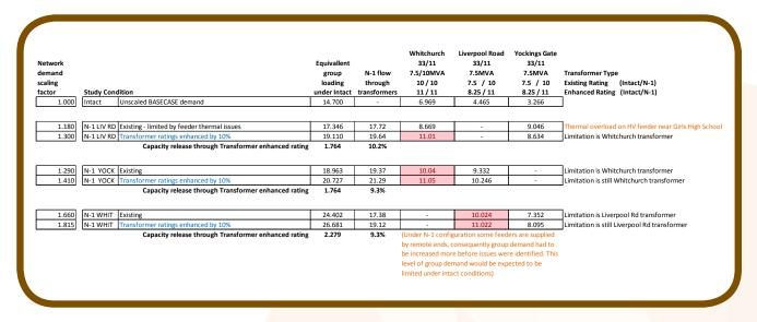
For all three transformer outage conditions studied, enhancing the rating of the transformer by 10% released significant amounts of capacity.
