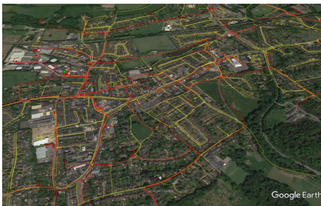
Figure 7 – Example of a Global Earthing System (GES)
