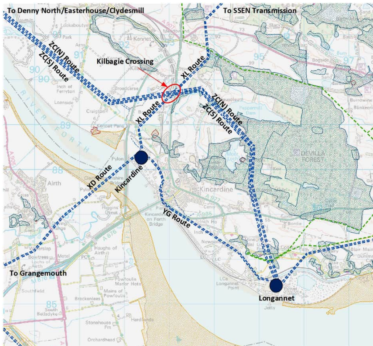
Figure 1: Existing SPT network around Kincardine area
