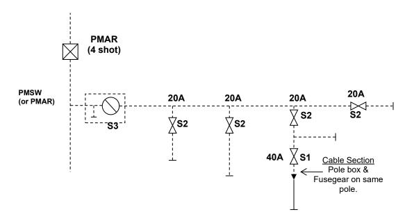
Where the design of a three-phase spur necessitates the use of 63A, or 100A ASLs, a PMSW / PMAR, shall be installed where practicable. If the network lends itself to further treatment, then consideration should be given to the use of additional 20A 2-shot ASLs for sub-spur sectionalising.
