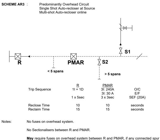
>5 spans in length. In this situation, source SEF protection should be set to 15 seconds.
