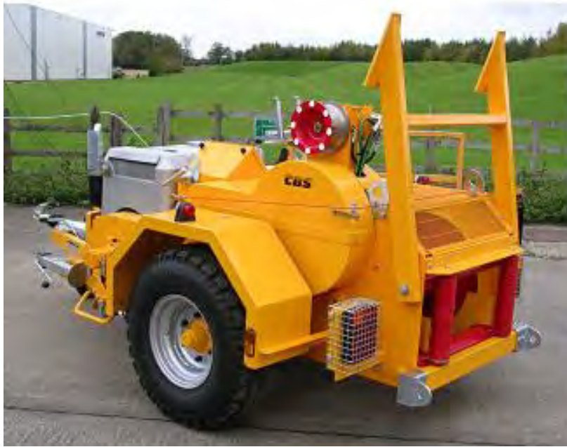
Plate 12: A typical pulling winch
