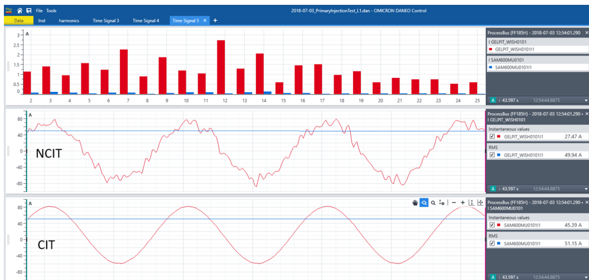
Figure 79. LPIT has higher accuracy measurements at lower magnitude levels
