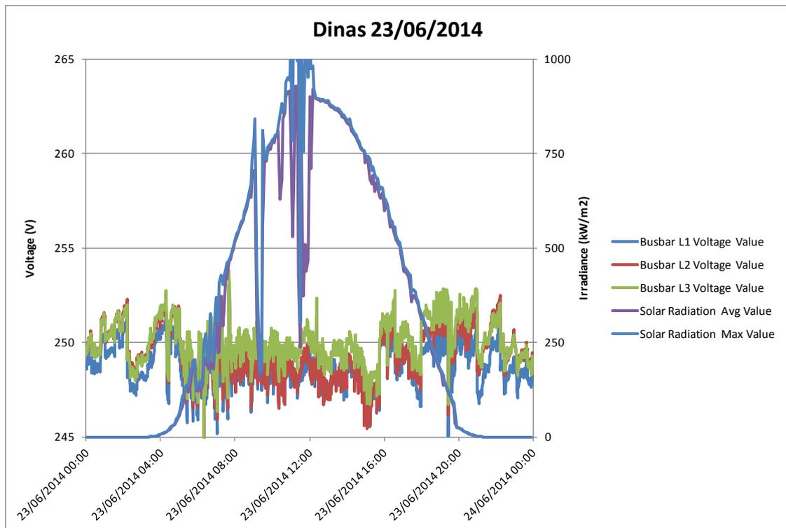
Figure 5-3 Dinas Measured Voltage and Solar Irradiance (23/06/2014)
