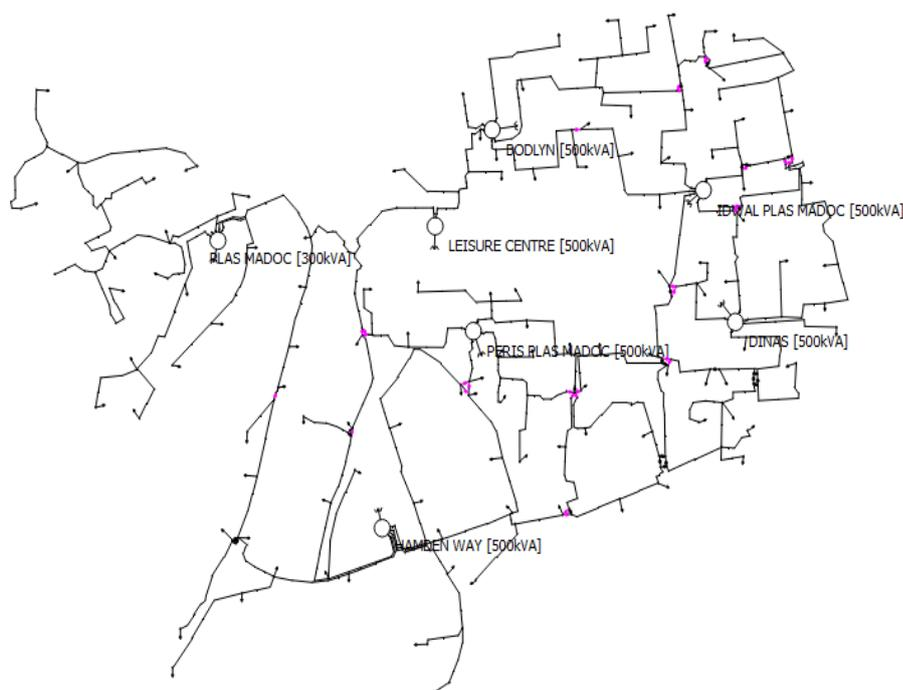
Figure 3-1 IPSA Model of the Ruabon LV Network Analysed (link boxes shown in pink)
