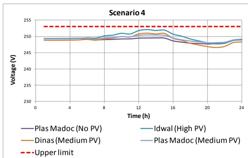
Figure 4-1 Voltage Profile for Scenario 4
