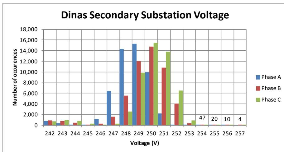
Figure 5-6 Voltage Distribution at Dinas Secondary substation
