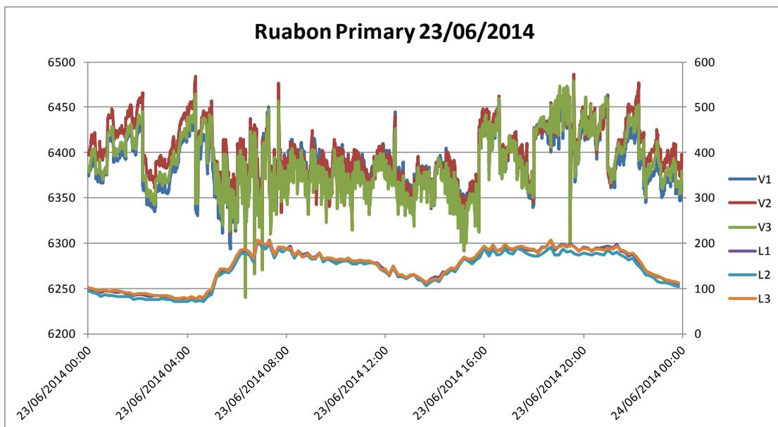
Figure 5-5 Ruabon Primary Measured Phase Voltage and Current (23/06/2014)
