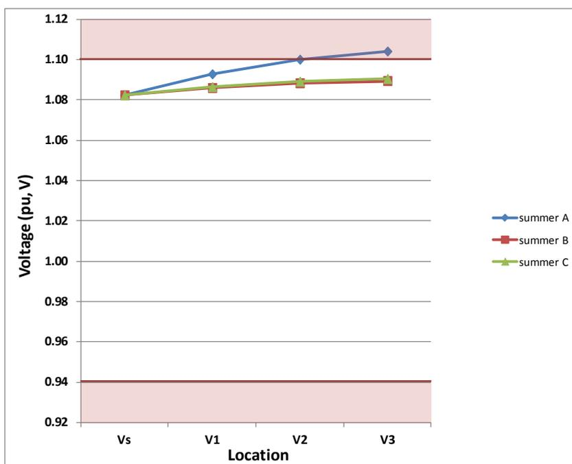
Figure 3-9 Voltage Along LV Feeder, Unbalanced Demand/Generation Case
