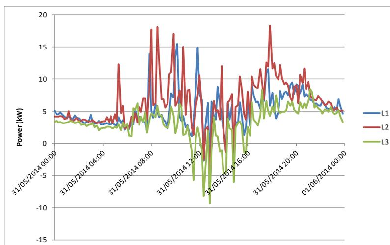
Figure 3-7 Power Profile of Typical LV Feeder at Secondary Substation showing Generation Phase Imbalance on High Solar Irradiance Day
