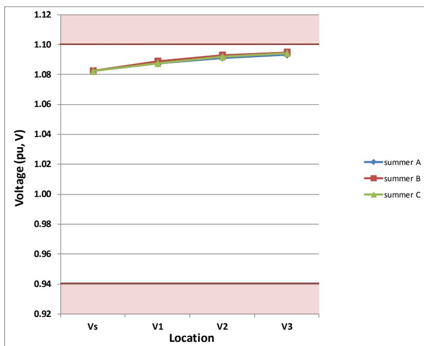
Figure 3-8 Voltage Along LV feeder, Balanced Demand/Generation Case
