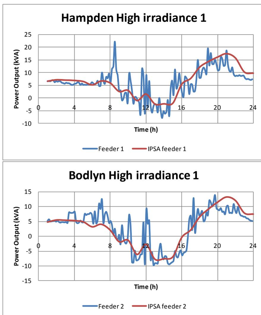
Figure 3-11 Validation of LV Feeder Modelled and Measured Loads
