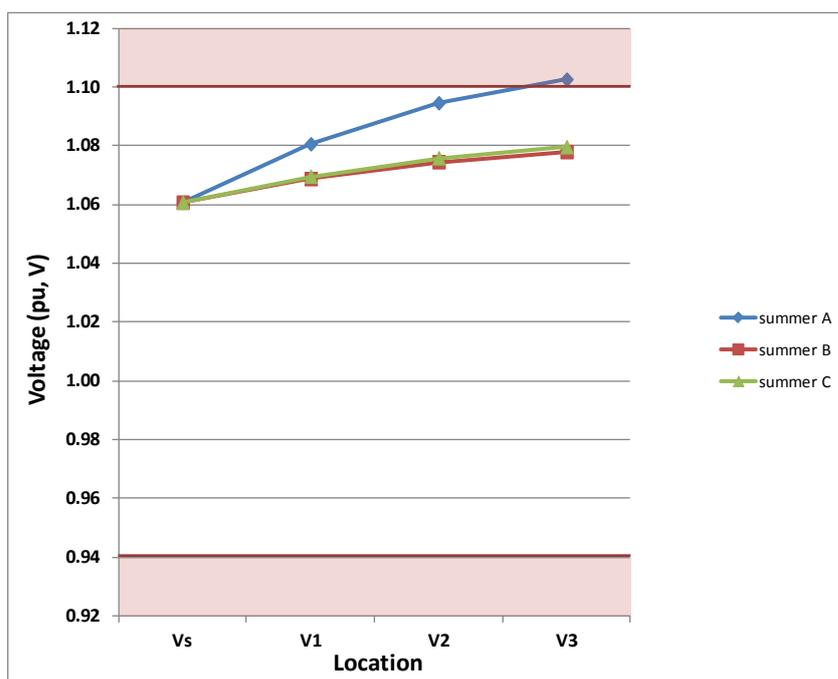
Figure 3-10 Voltage Along LV Feeder, Unbalanced Demand/Generation Case with 2% Voltage Reduction)
