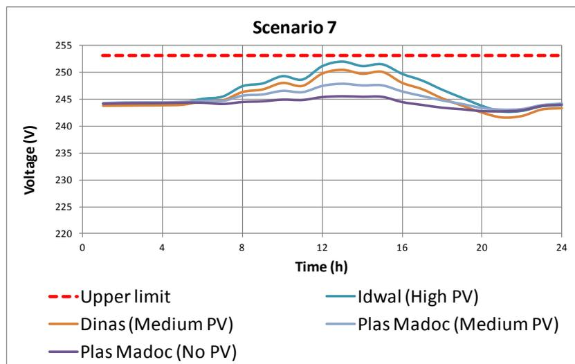
Figure 4-4 Voltage Profile for Scenario 7
