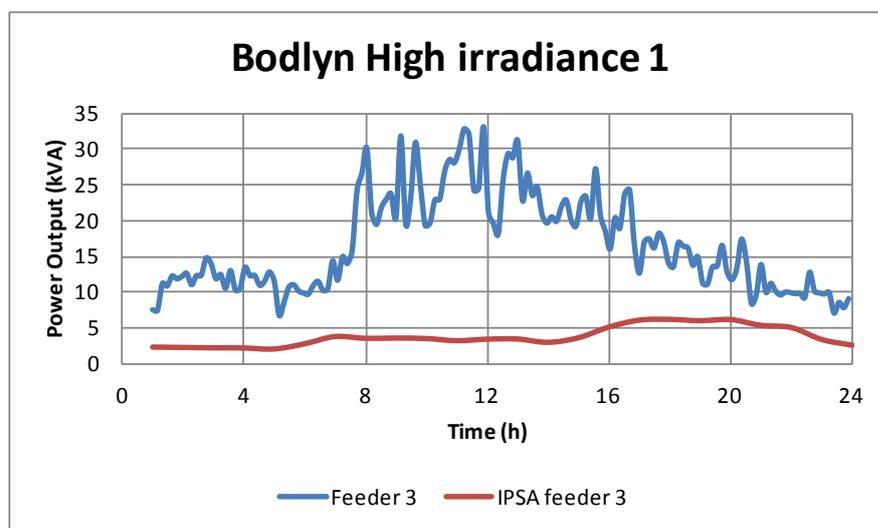
Figure 3-12 Validation of LV Feeder Modelled and Measured Loads (with high commercial demand)
