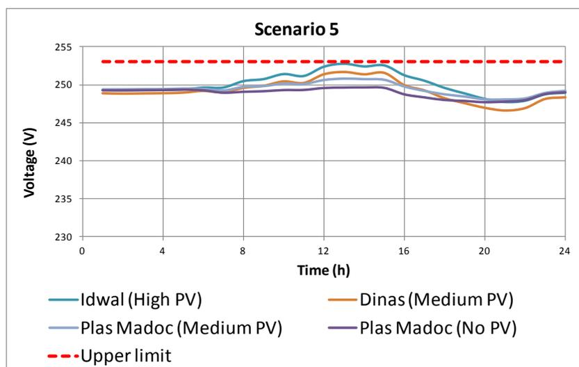
Figure 4-2 Voltage Profile for Scenario 5
