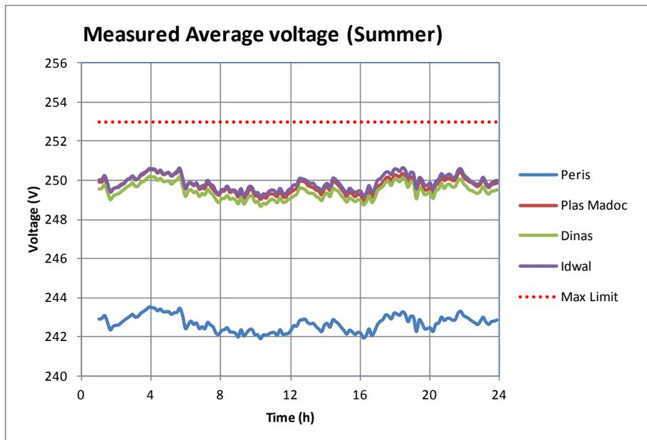
Figure 5-1 Measured Average Voltage
