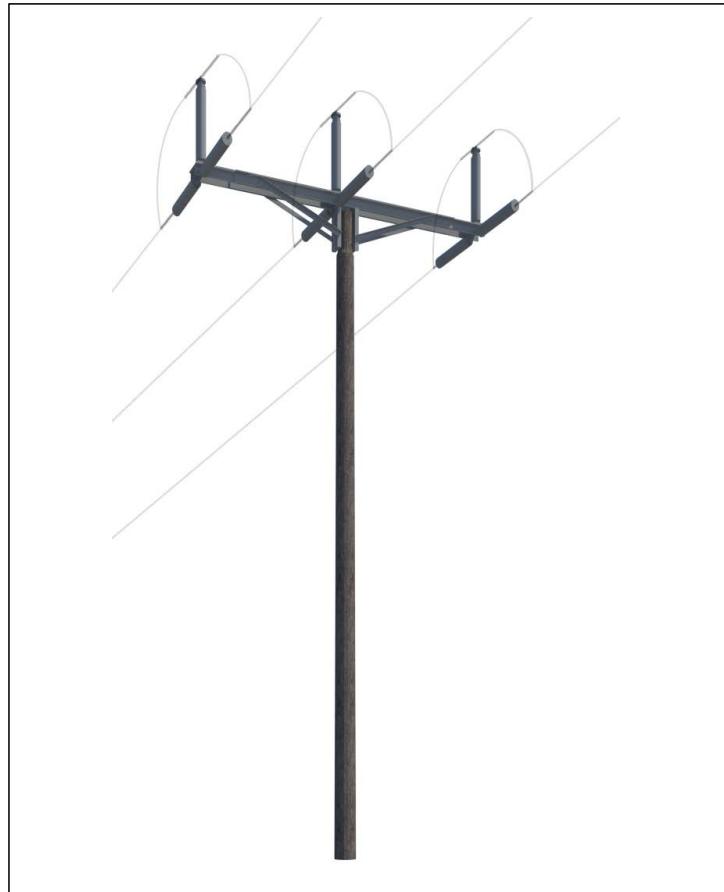
Component parts of 132kV 'Trident' design wood pole: Angle
