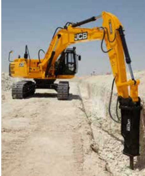
Figure 32 Excavator fitted with a hydraulic breaking attachment
