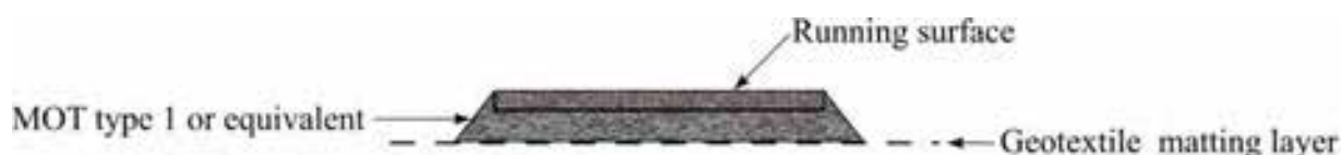
Figure 13 Typical haul road construction detail
