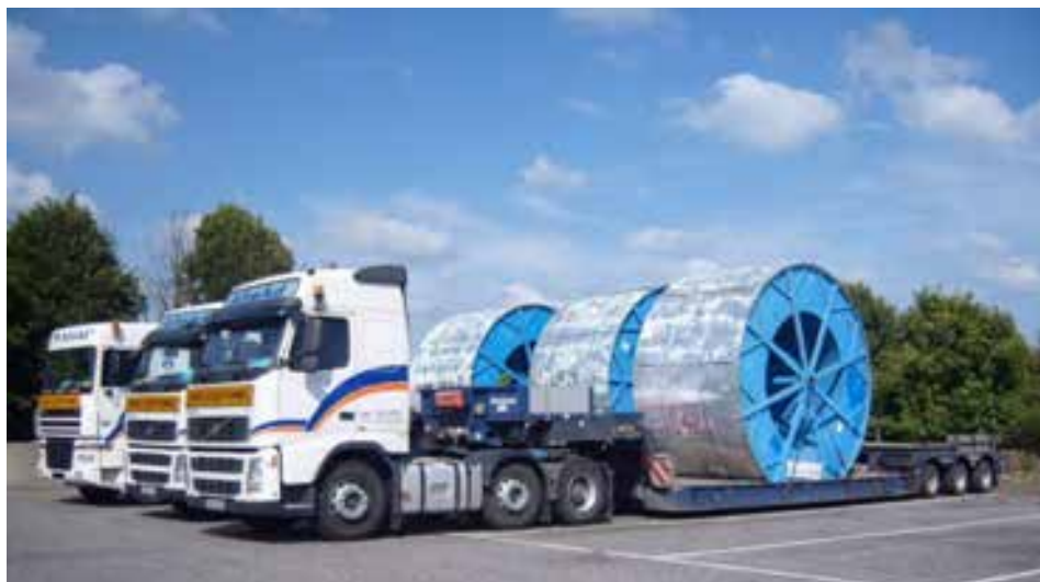
Figure 19 Cable drum on a low loader trailer
