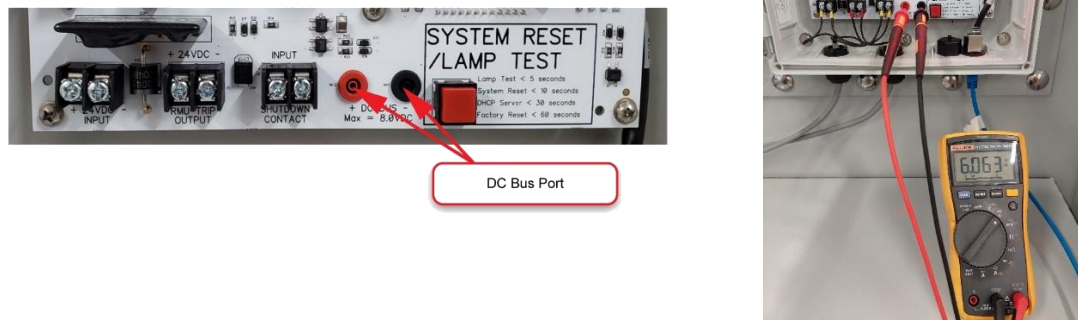
Figure 18 – Measuring the internal stored energy of the UPFC via the DC Bus Port
