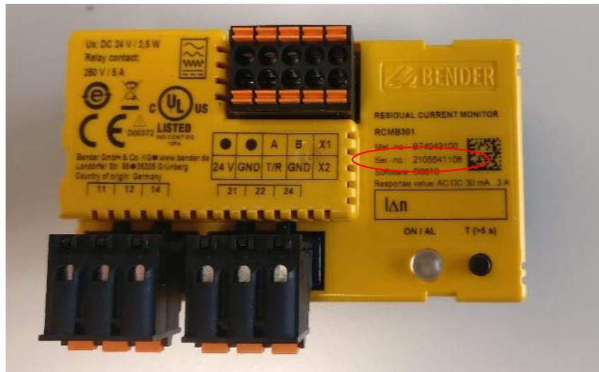
**Figure 74 – Bender RCMB301 serial number location**
