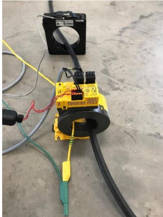
**Figure 71 – USB interface with Bender RCMB301**
