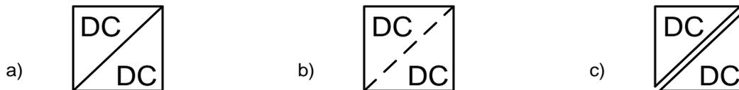
**Figure 2.9 DC-DC converter symbols: (a) DC-DC converter, (b) non-isolated DC-DC converter, (c) isolated DC-DC converter.**
