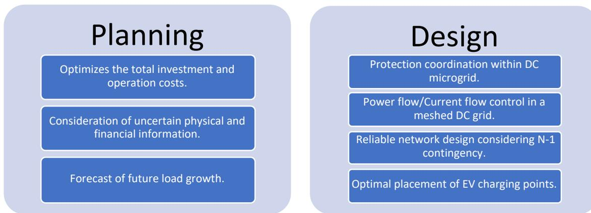
Figure 2.10 Key requirement to be considered when planning and designing a DC microgrid.
