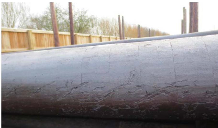
Wood Poles With Preservative Creosote
