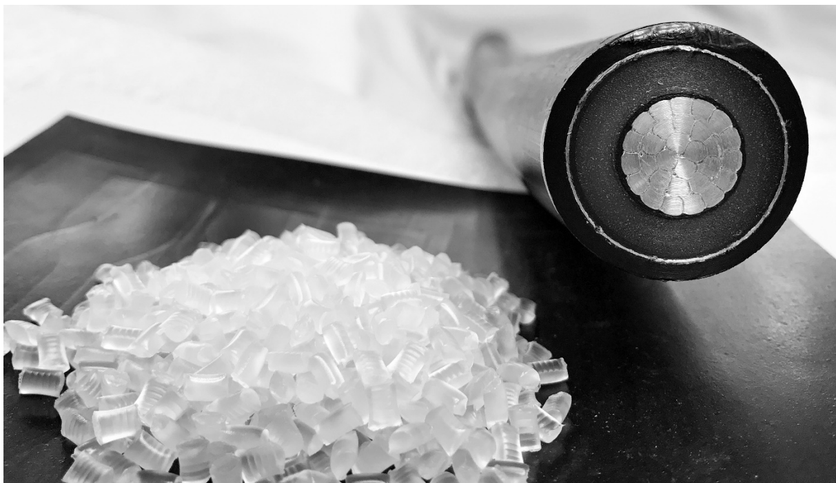
Figure 11 Picture showing the pelletised blend granules which are translucent with the corresponding extruded MV cable. The aluminium conductor has an adjacent black inner semiconducting screen and there is an outer screen bounding the insulation layer – this layer appears dark grey because the cross section acts as a black reflector.
