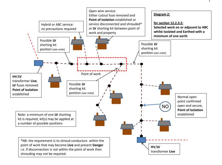
The following categories of work may be carried out with the conductors **Isolated** and **Earthed** with a minimum of one earth, but not **Earthed** in accordance with 12.2.3.3 below.
