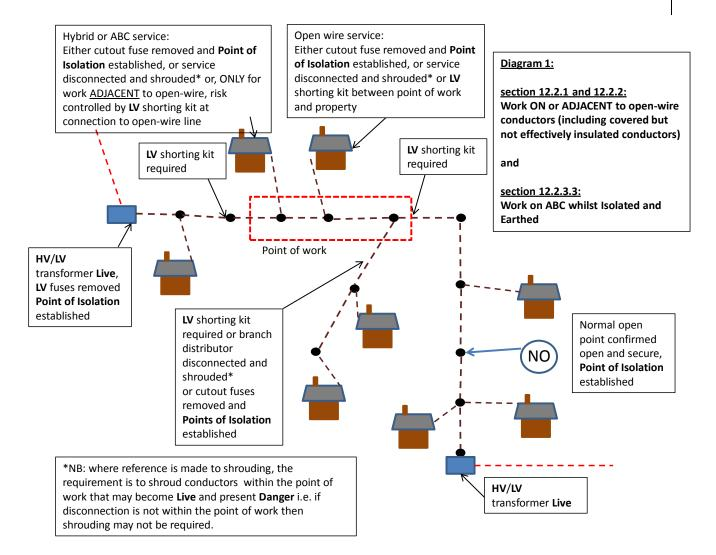
12.2.2 Work on or adjacent to **Isolated** covered but not effectively insulated conductors in an openwire configuration (see Diagram 1)
