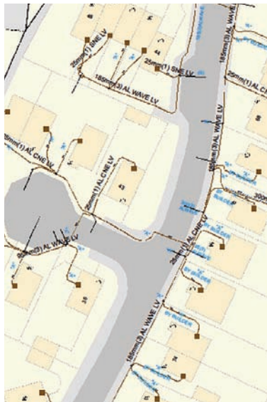
Example of SP Energy Networks cable records highlighting cable routes
