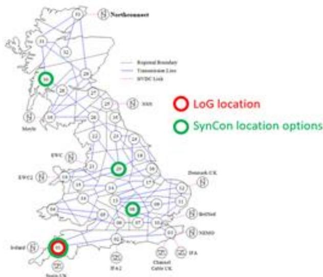
Figure 16: GB transmission network illustrating locations of LoG and SC for Scenario 1.
