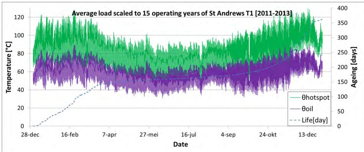
**Figure 6-1: Temperature profiles with a peak loading of 30,4 MVA to reach a maximum lifetime of 15 years**
