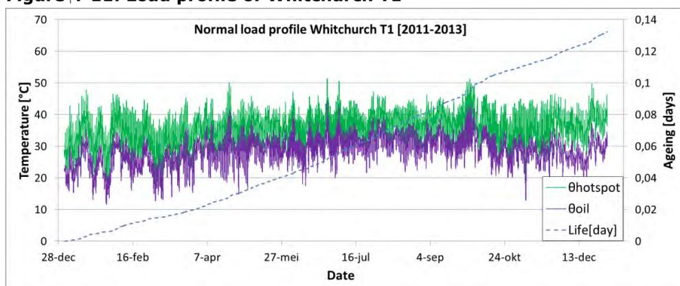
Figure 4-12: Hot-spot and oil temperature profile and ageing as function of time of transformer T1 at substation Whitchurch, based on the ambient temperature and averaged load profile
