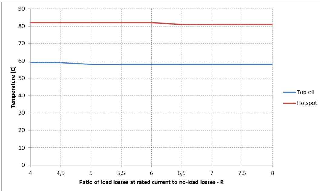
**Figure 7-3: Top oil temperature and hot spot temperature as function of the ratio of load losses at rated current to no-load losses**
