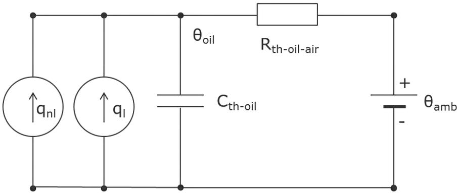
**Figure B-3: Thermal model used in IEC 60076-7**
