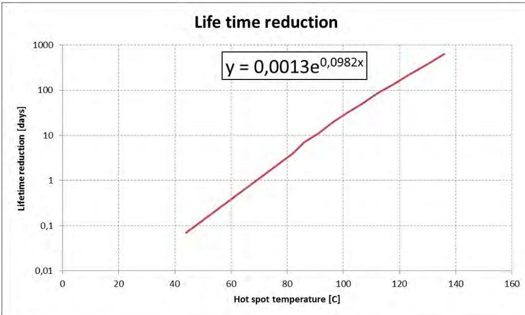
**Figure 7-5: Life time reduction as function of the hot spot temperature**
