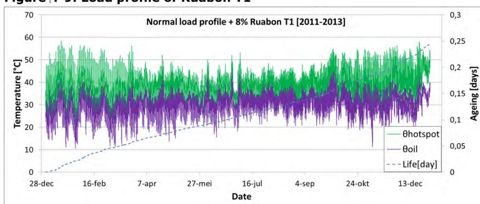
Figure 4-10: Hot-spot and oil temperature profile and ageing as function of time of transformer T1 at substation Ruabon, based on the ambient temperature and averaged load profile
