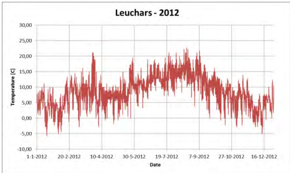
**Figure 3-1: Ambient temperatures profile the transformers St. Andrews T1, St. Andrews T2, Cupar T1 and Cupar T2.**
