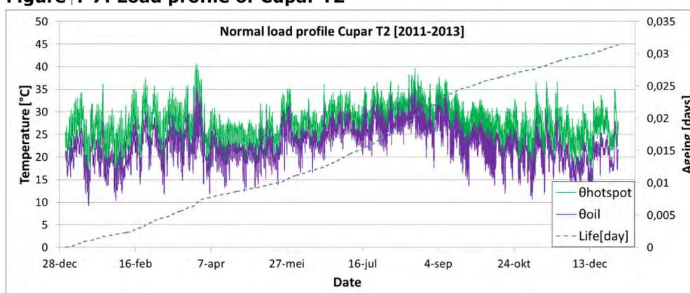
**Figure 4-8: Hot-spot and oil temperature profile and ageing as function of time of transformer T2 at substation Cupar, based on the ambient temperature and averaged load profile**
