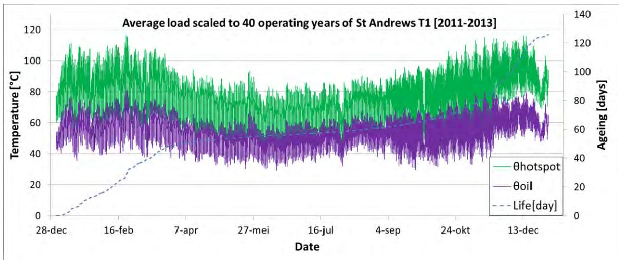
**Figure 6-2: Temperature profiles with a peak loading of 28,1 MVA to reach a maximum lifetime of 40 years**
