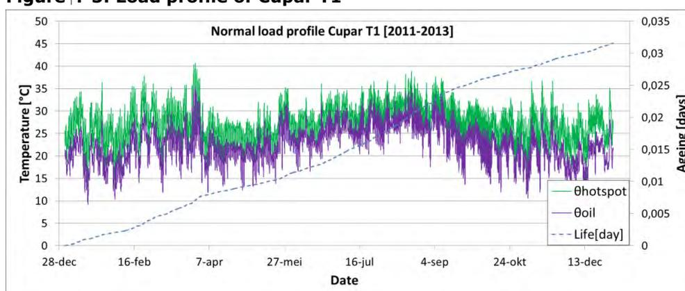
**Figure 4-6: Hot-spot and oil temperature profile and ageing as function of time of transformer T1 at substation Cupar, based on the ambient temperature and averaged load profile**
