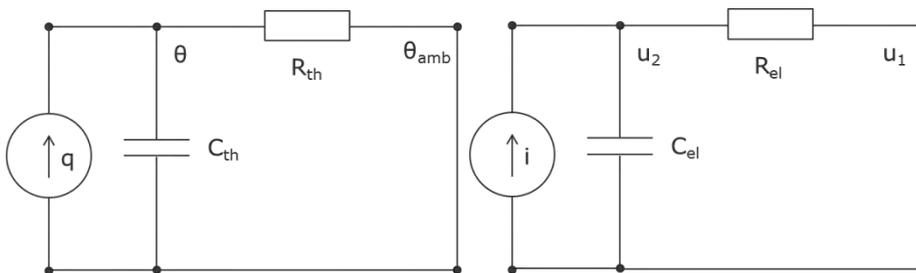
**Figure B-2: Thermal transformer model (left) and its electrical analogue (right)**
