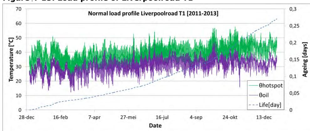
Figure 4-16: Hot-spot and oil temperature profile and ageing as function of time of transformer T1 at substation Liverpoolroad, based on the ambient temperature and averaged load profile
