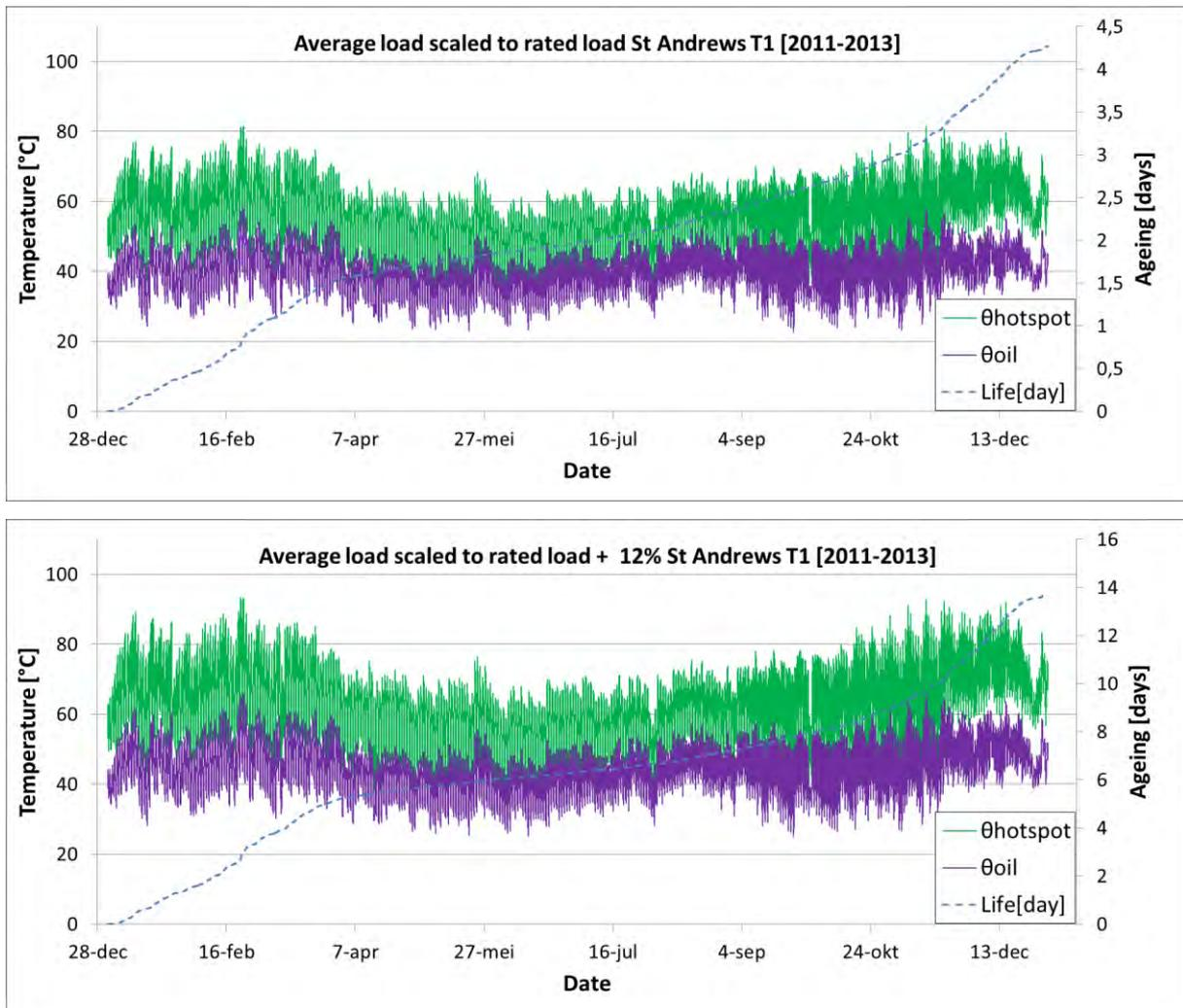
**Figure 5-2: Temperature profiles with a peak loading of 21 MVA (top) and 21 MVA + 12% (bottom) without exceeding a hot-spot temperature of 98 °C**
