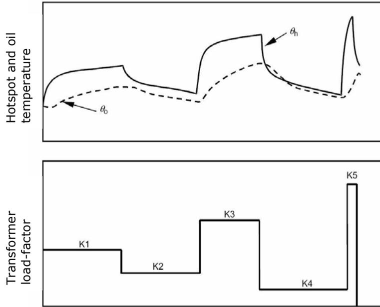
**Figure B-4: Temperature responses to step changes in the load current (in which K1 till K5 are different load-factors) /1/**
