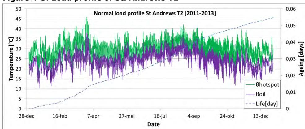
Figure 4-4: Hot-spot and oil temperature profile and ageing as function of time of transformer T2 at substation St. Andrews, based on the ambient temperature and averaged load profile
