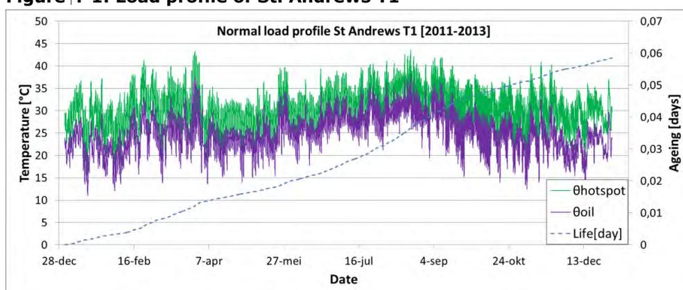
Figure 4-2: Hotspot and oil temperature profile and ageing as function of time of transformer T1 at substation St. Andrews, based on the ambient temperature and averaged load profile
