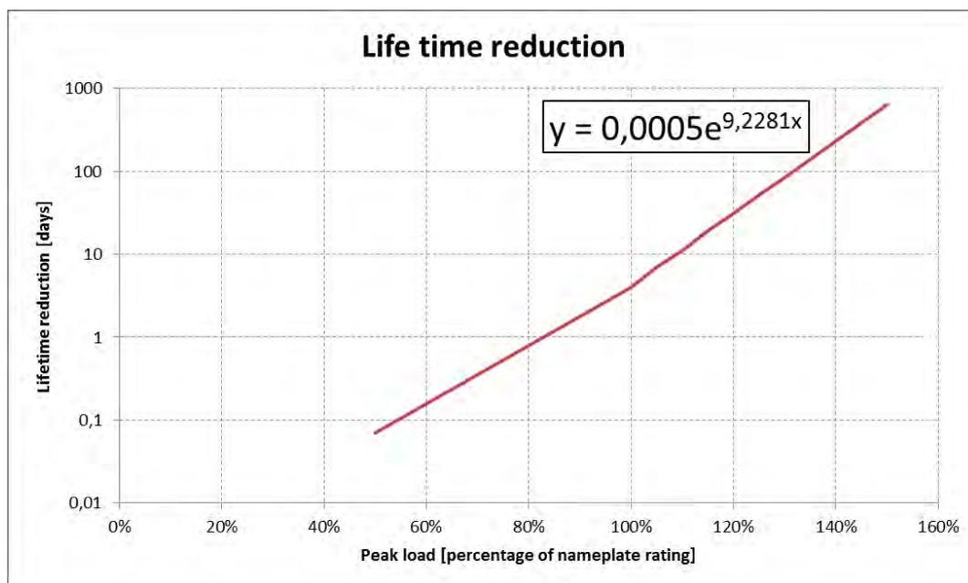
Figure 7-4: Life time reduction as function of the peak load
