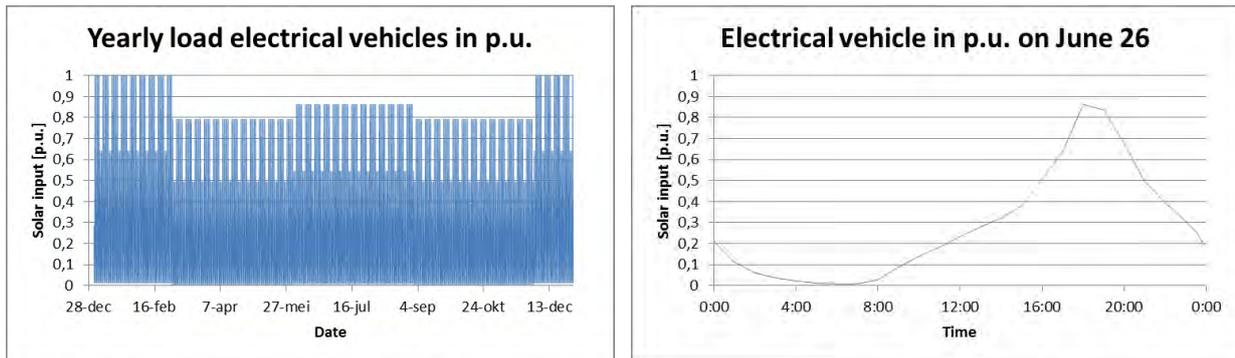
**Figure 8-3: Examples of load patterns of electrical vehicles per year (left) and on June 26 (right)**
