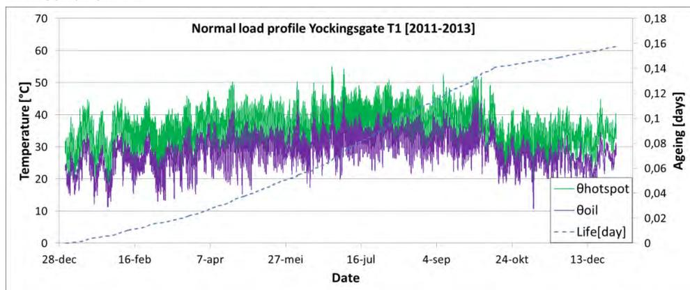
**Figure 4-14: Hot-spot and oil temperature profile and ageing as function of time of transformer T1 at substation Yockingsgate, based on the ambient temperature and averaged load profile**
