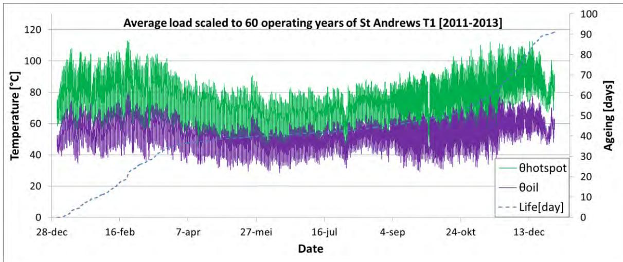
**Figure 6-3: Temperature profiles with a peak loading of 27,5 MVA to reach a maximum lifetime of 60 years**
