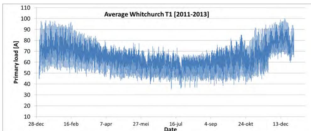
Figure 4-11: Load profile of Whitchurch T1
