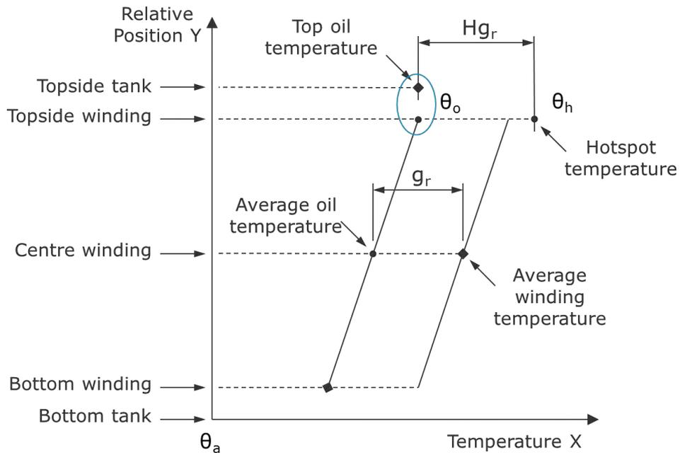
**Figure B-1: Thermal diagram**
