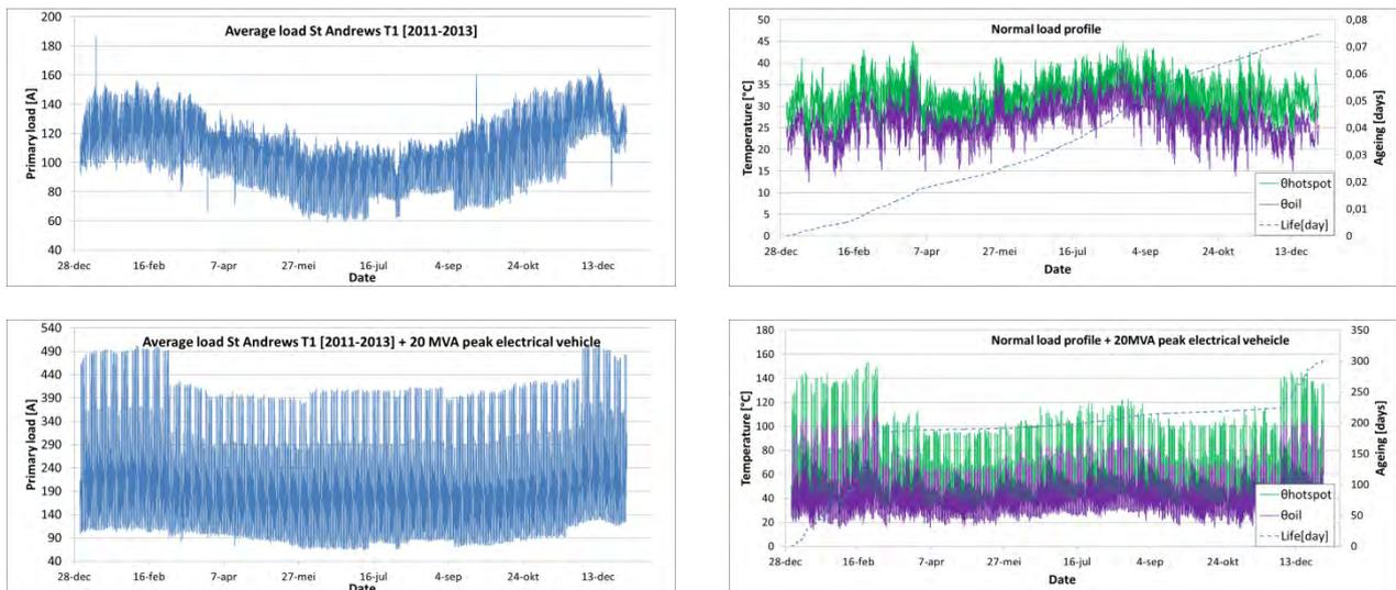
Secondly, additional loading due to charging of electrical vehicles of 5, 7.5, 10 and 12.5 MVA has been superimposed on the load profile which has already been artificially increased to a peak power of 21 MVA. Below the simulation results for the 21 MVA load profile and the 12.5 MVA profile are shown.
