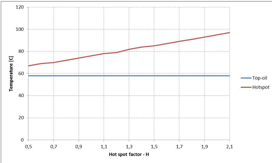
**Figure 7-2: Top oil temperature and hot spot temperature as function of the hot spot factor**
