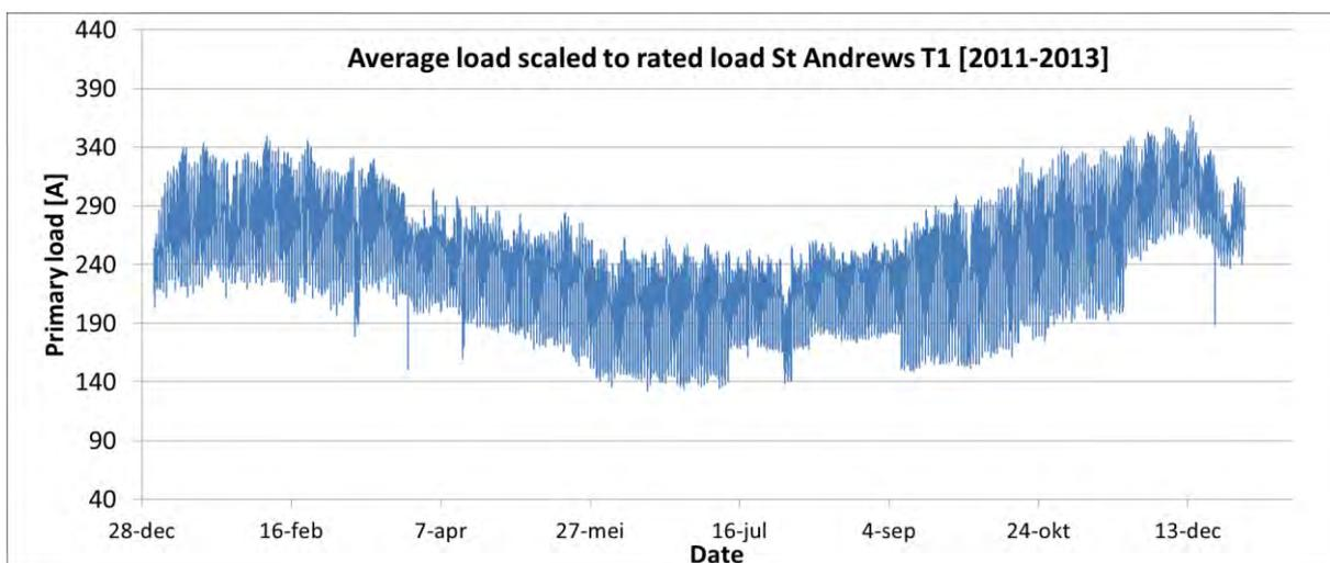
**Figure 5-1: Artificial load profile increased to rated peak load based on actual load pattern**
