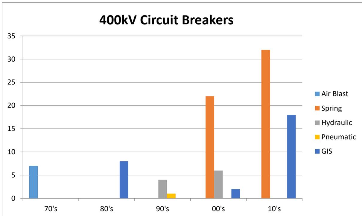
Figure 3: 400kV CB by Type Overview Installations in SPT Transmission Network.
