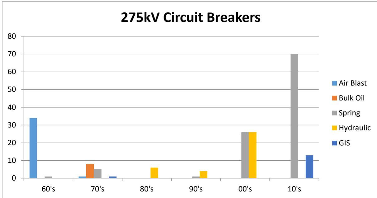
Figure 2: 275kV CB by Type Overview Installations in SPT Transmission Network.
