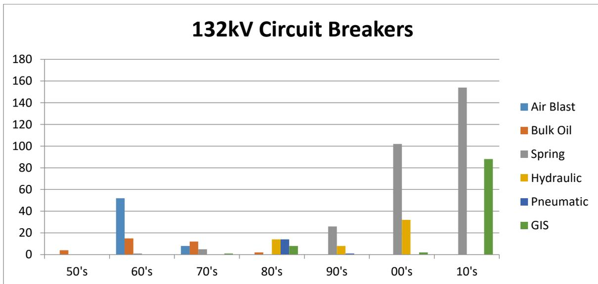
Figure 1: 132kV CB by Type Overview Installations in SPT Transmission Network.
