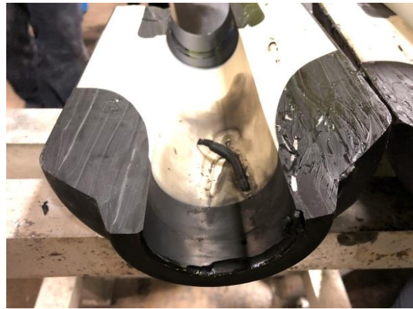
Figure 6: post-mortem termination inspection.
