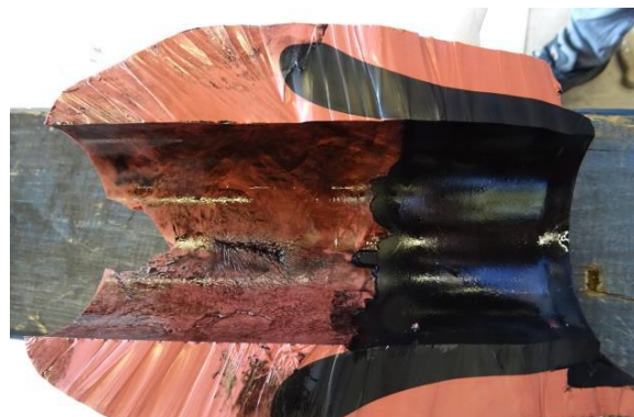
Figure 10: post-mortem termination inspection.
