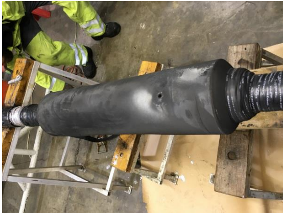
Figure 7: post-mortem termination inspection.
