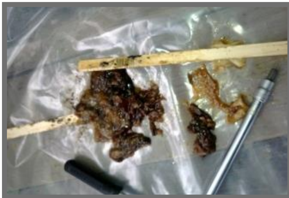
Figure 1 (Meadowhead): oil contamination March 16.
