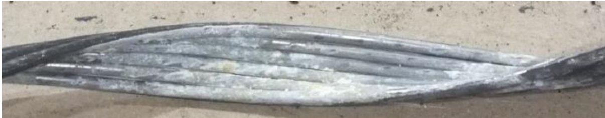
Figure 1: inner aluminium strands exhibit a significant level of aluminium corrosion product.
