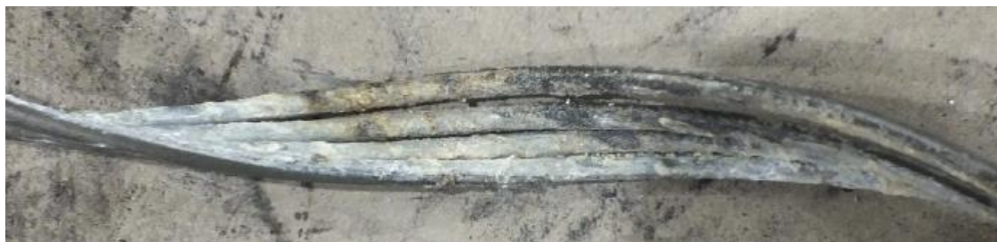
Figure 1: inner aluminium strands exhibit a significant level of aluminium corrosion product.
