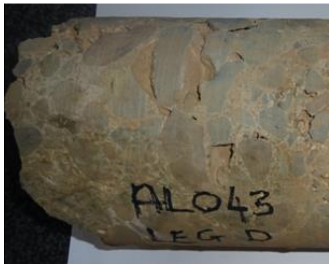
Concrete core sample
