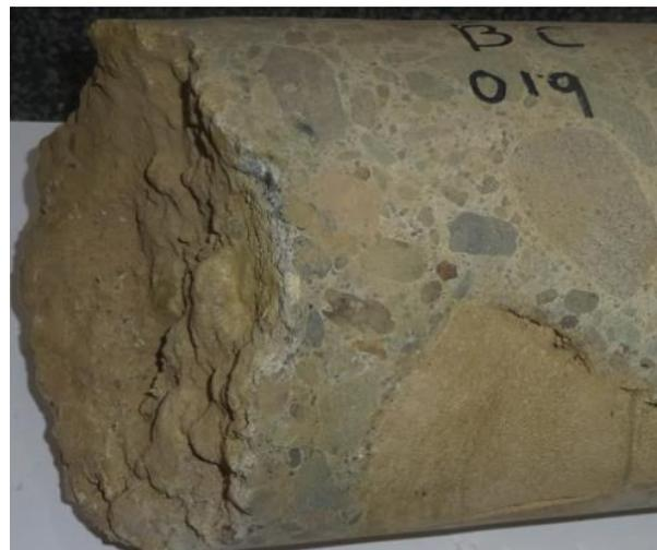
Concrete core sample tower BC019
