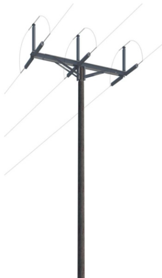
Component parts of 132kV 'Trident' design wood pole: Angle
