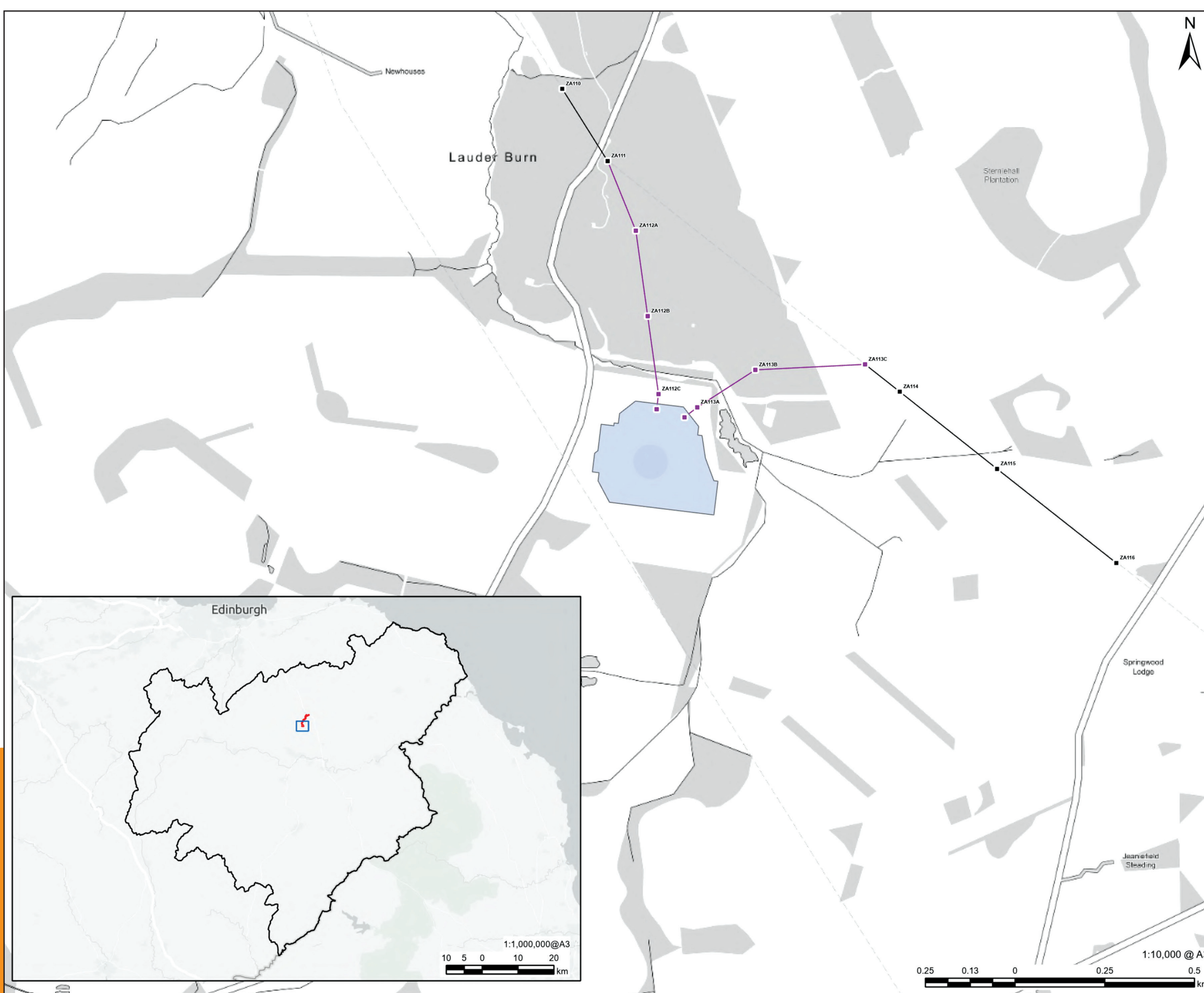
Figure: ZA overhead line diversion location plan
