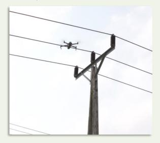
Figure 14 Use of drones for overhead line assessment
